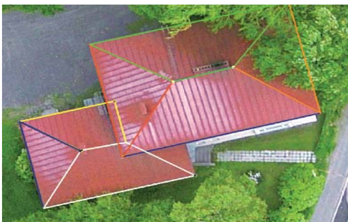
Planar surfaces of roofs can be detected from laser points. Their edges can be edited only manual by using 'bird-eye view' and raw images as reference.
